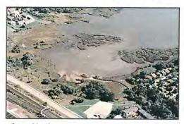
Figure 16. View over northern part of Frenchman's Bay showing large mudflat area derived from sediment-laden urban runoff from Amberlea and Dunbarton creek catchments (Fig. 6). As recently as 1972, the northern part of the bay was continuous wetland (Fig. 14).
